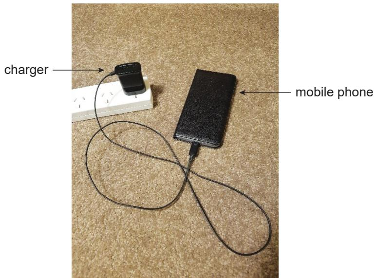
The transformer decreases the voltage from 220 V to 5.0 V. The primary coil of the transformer has 3520 turns.
