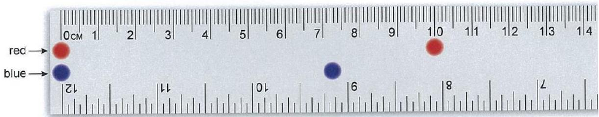
The ruler was placed 50 cm from the diffraction grating, as shown in the diagram below.
