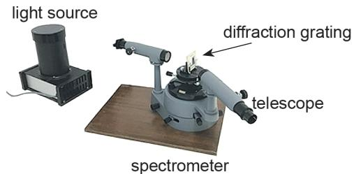
The student observes the zero-order maximum of the spectrum when the telescope is at **A**, at an angle of  $0^\circ$ . The student then moves the telescope from **A** until the first-order maximum is observed, when the telescope is at **B**, at an angle  $\theta$  of  $15.4^\circ$ , as shown in the diagram below.
