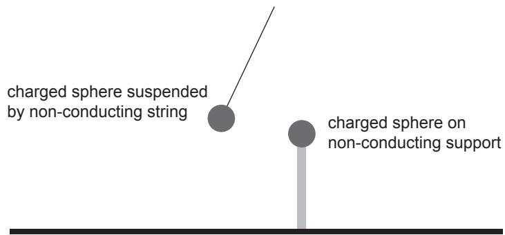
The two spheres each have a charge of  $+3.4 \times 10^{-9}$  C, and the distance between each of their centres is 3.2 cm.
