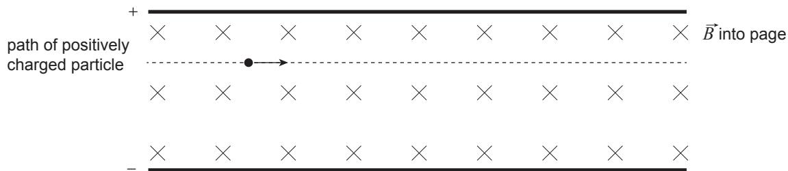
The diagram shows the path of a positively charged particle that has entered the fields at speed  $v$ , perpendicular to each field. The particle passes through the fields without being deflected.
