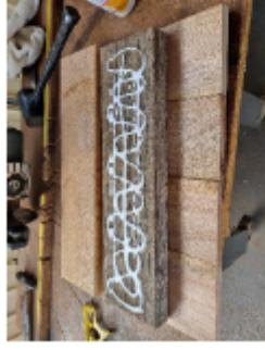
I then begin gluing 7 pieces of scrap pine to from what will be the main seat component using PVA wood glue.
