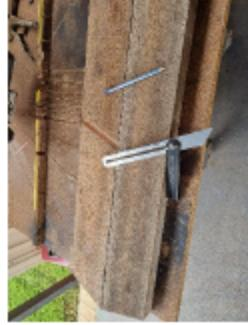
Next, I am once again using the chisel to create another rebate in a different position on the legs this time. This 30 degree chiselled rebate allows the main seat component to slide in being sturdy and/or reliable.
