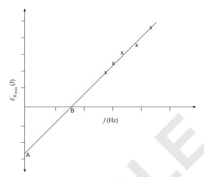
The line of best fit intersects the  $E_{K_{\rm max}}$  axis at A and the f axis at B.
