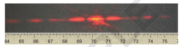
(a) Determine the distance between adjacent maxima in the interference pattern  $\Delta y$  for the image above.
